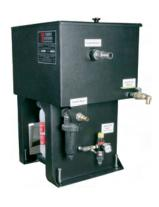
Unlike competitive belt and wheel skimmers, the PhaSep draws coolant into the coalescing box at a minimum rate of 1,000 gallons per day. Frequent tank volume turnover guarantees oil removal. The Tri-Ball Float captures the oil where it accumulates most, at the surface of the coolant. A simple weir dam arrangement captures the oil and sends it to a holding tank for disposal. Clean coolant is gravity fed back to the machine
